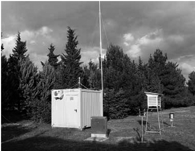
Figure 2: The continuous PM10 particulate monitoring station (TEOM 1400A) in the Port of Koper Slika 2: Stalna postaja za spremljanje suspendiranih delcev (TEOM 1400A) v Luki Koper
